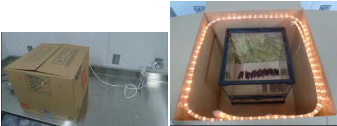
Figure 65: Enclosure for the pupae: (Left) Closed box creates day/night conditions with a timer controlling the LED lights, shown in part (Right)
